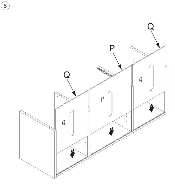
6, Attach thin back, board (Q, P) to the TV cabinet body.
